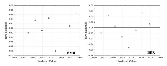
Figure 2. Residue versus the predicted value from data specific gravity for BMR and BER.
