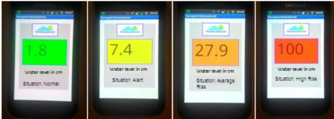
Figure 7: The functioning of Nimbusdroid application on a mobile device
