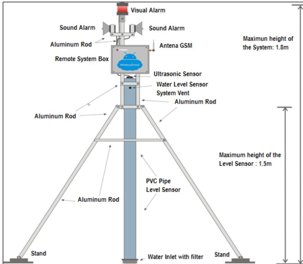
Figure 5: Side view of Nimbusdroid equipment
