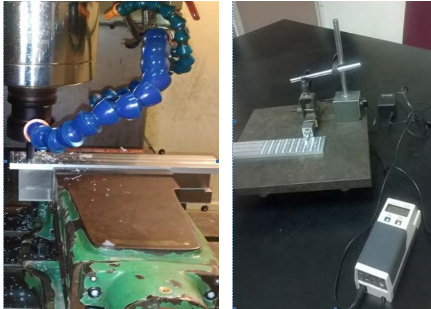
Figure 1: Experimental setup, Measurement of surface roughness using Surf Test-211 series
