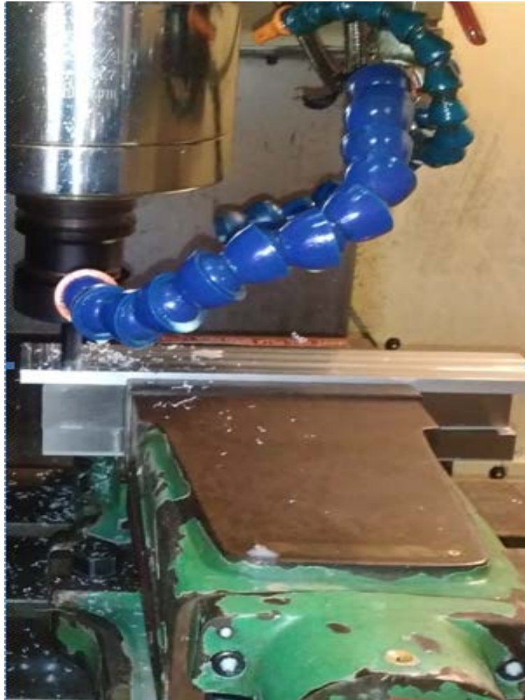
Figure 1: Experimental setup (CNC Vertical Machining Center, KENT INDIA Co, Ltd, Taiwan)
