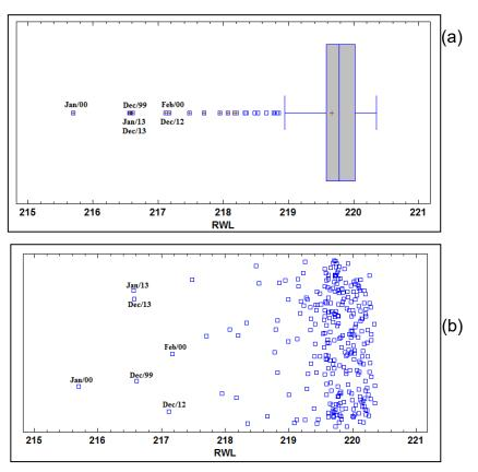
Figure 3: (a) Box-Plot and (b) Scatterplot graphic of the reservoir water level (RWL) from Itaipu dam, from Jan /90 to Dec /13
