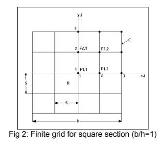
From Prandtl's analogy, the stress function at boundary shown in figure 2 is zero and exists throughout the region R shown in figure 2 except at the boundary.
