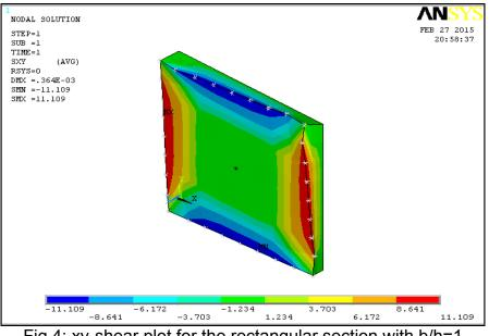
Fig 4: xy-shear plot for the rectangular section with b/h=1
