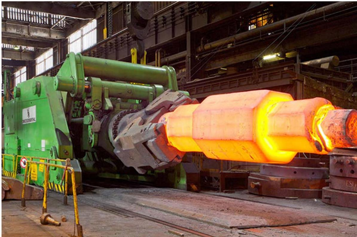
Figure 1: A railbound forging manipulator
