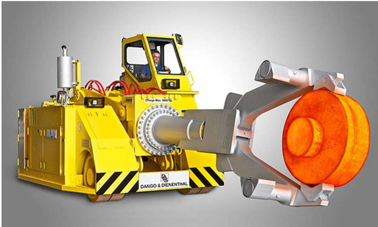
Figure 2 A mobile forging manipulator
