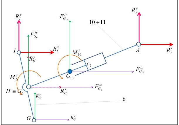
Figure 6: The forces schema of the dyad 6,10-11
