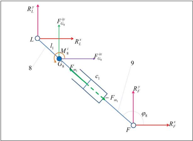
Figure 9: Forces schema of the motor mechanism c1
