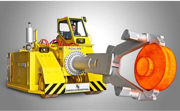
Figure 2 A mobile forging manipulator Source: Dango and Dienenthal
