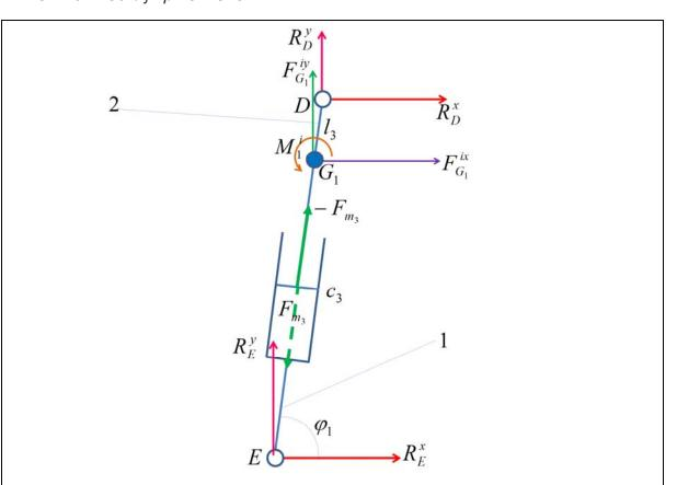
Figure 11: Forces schema of the motor mechanism c3
