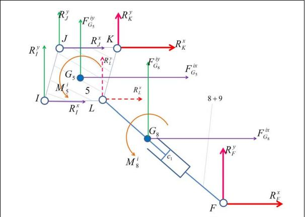
Figure 8: The forces schema of the dyad 5,8-9
