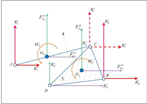
Figure 7: The forces schema of the dyad 3,4
