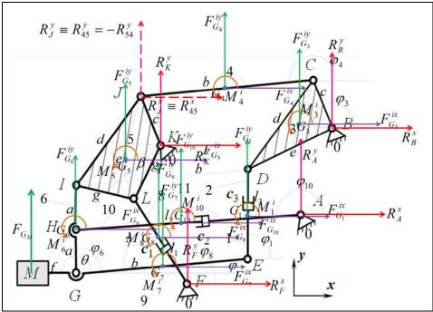
Figure 4: The forces schema of the main mechanism
