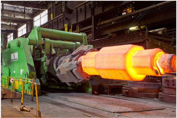
Figure 1: A railbound forging manipulator Source: Dango and Dienenthal
