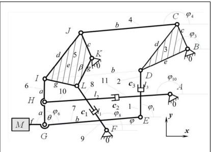
Figure 3: The kinematic schema of the main mechanism
