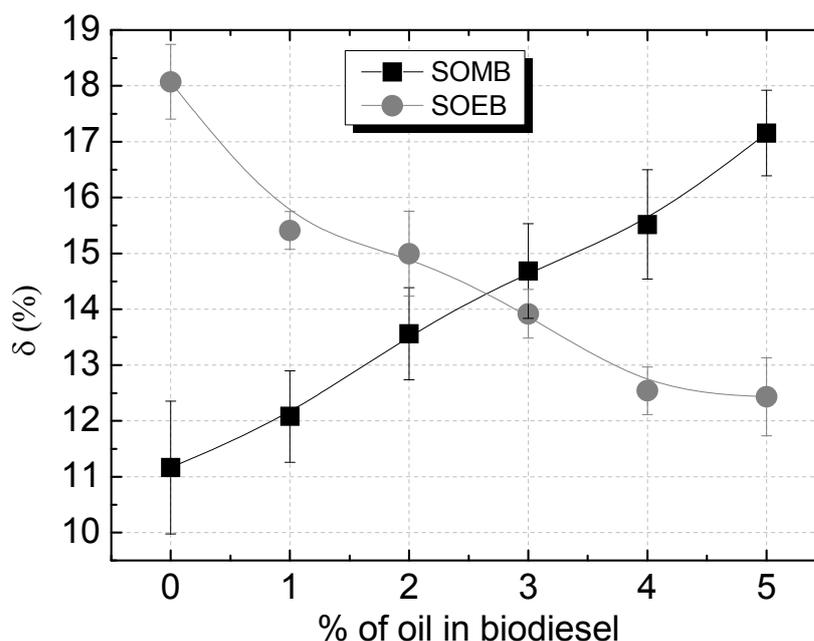
Figure 4.  $\delta = [(I_{1096} - I_y) / I_{1096}] \times 100\%$ , with  $I_{1096}$  corresponding to the absorption intensity of soybean oil and biodiesel, and  $I_y$  representing the absorption intensity in  $y = 1017 \text{ cm}^{-1}$  for MB and  $y = 1035 \text{ cm}^{-1}$  for EB.
