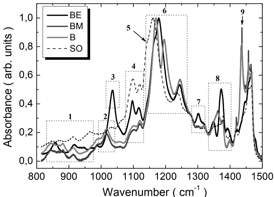
Figure 1. Absorption spectra in the fingerprint region of the samples of soybean oil (SO), ethylic biodiesel (EB), methylic biodiesel (MB) and commercial biodiesel (B).
