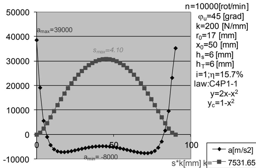
Figure 4. The dynamic analysis of the new law, C4P, Module C,  $\varphi_u=45^\circ$ ,  $n=10000$  rpm
