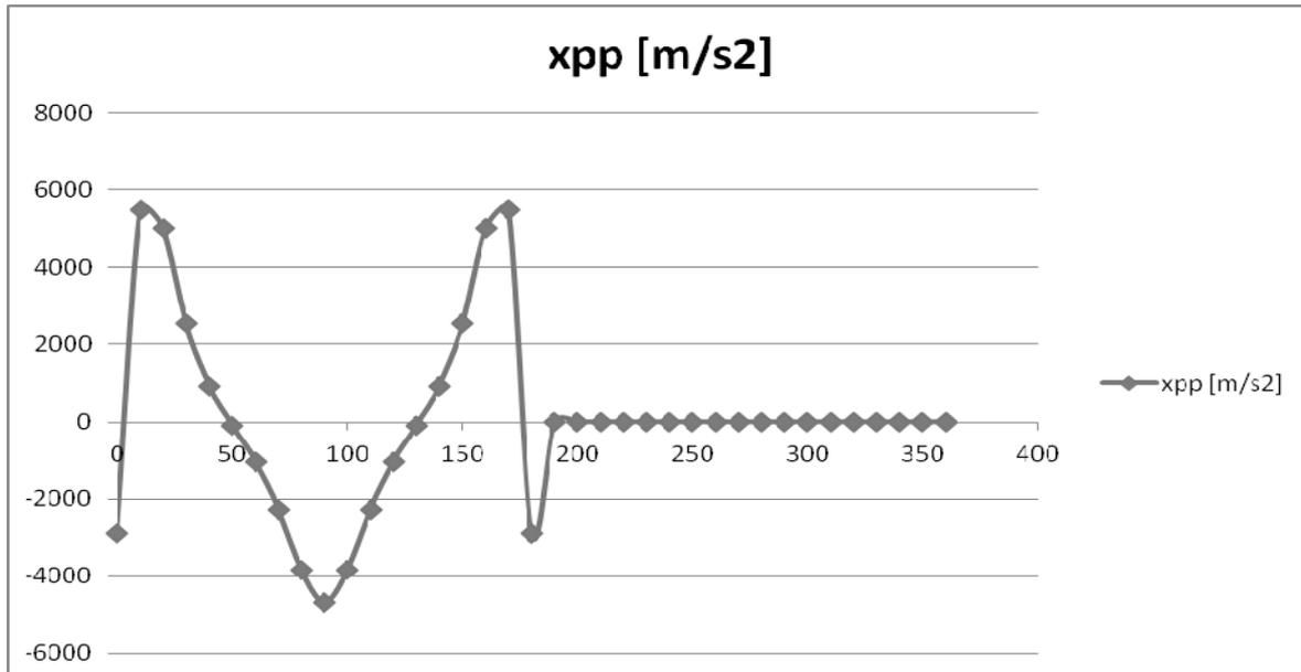
Figure 9. The dynamic diagram at the cosine profile at the cam with translated follower with roll;  $r_0=13$ [mm];  $h=20$ [mm];  $\varphi_u=\pi/3$ [rad];  $r_b=2$ [mm];  $e=0$ [mm];  $n=5500$ [rpm];  $x_0=9$ [cm];  $k=500$ [kN/m]
