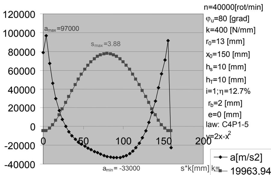
Figure 5. Law C4P1-5, Module B,  $\varphi_u=80^\circ$ ,  $n=40000$  rpm
