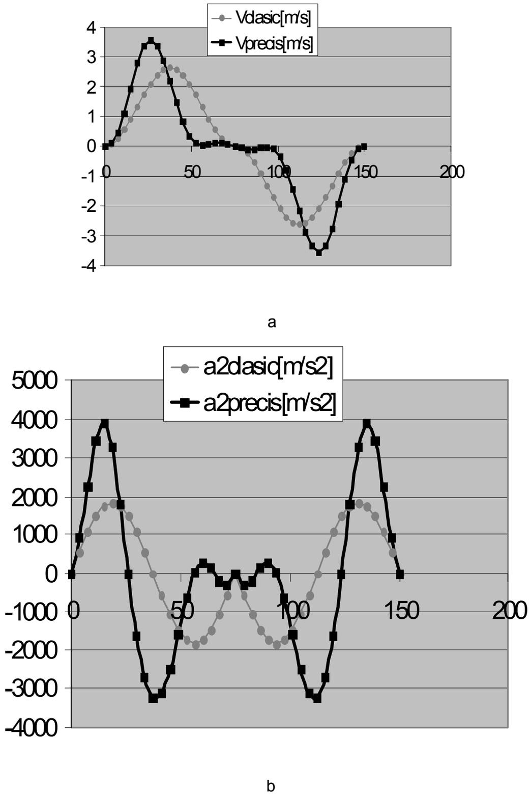
Figure 2. The classical and dynamic kinematics; a-velocities and b-accelerations of the follower
