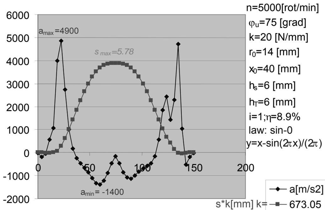
Figure 3. The dynamic analysis of the law sin, Module C,  $\varphi_u=75^\circ$ ,  $n=5000$  rpm
