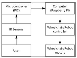
Figure 1: System's high level design
