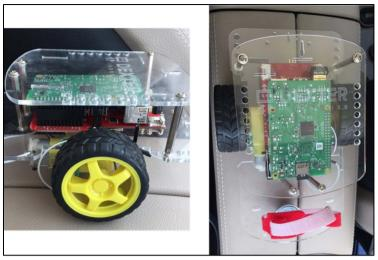
Figure 3: GoPiGo robot used in the prototype
