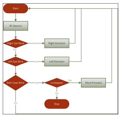
Figure 5: System's flowchart
